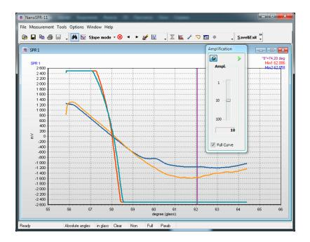
Increasing an amplification value is especially useful in the Slope mode (when the options 0 V left or 0 V right are selected), because this allows you to increase the sensitivity of the device multiple times. In Fig. is shown kinetics at amplification k = 10 for distilled water (n = 1.333) that was changed with saline (n = 1.337) in channel 1 and for diluted saline (n = 1.334...1.335) in the channel 2.
